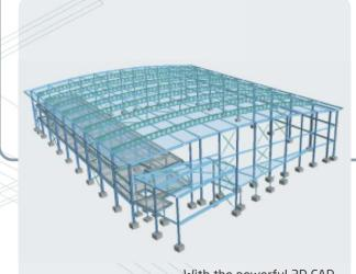
With the powerful 3D CAD packages the detailer can develop a building, as it would appear once built on site
